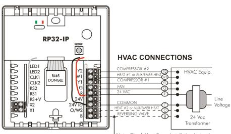
Note: Check Heat Pump Installation Instructions for reversing valve connection, either 'O' or 'B'.
