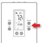
For UP32 and US32 thermostats, press the two buttons on the right side of the thermostat to activate the secondary display for remote sensors. Press the Up or Down buttons to cycle through the sensor types. Rotate through indoor, outdoor, humidity, and AUX1 on the display. There will be a value next to the icon for the sensor type that has been selected.
